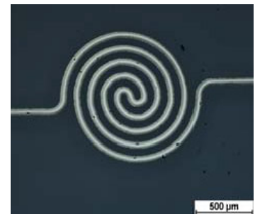
Fig. 2: Printed resistive temperature sensor
