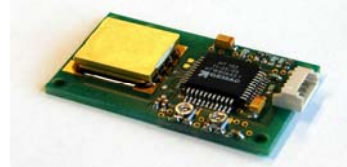
Fig. 3: MID-sensor on PCB
